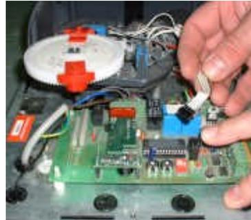
2. Pull back black retaining clip and remove limit switch cable.
