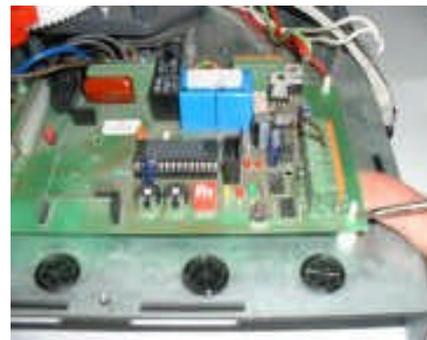
6. Using the screwdriver, press barb on PCB spacers (x5) and ease off PCB.
