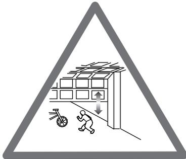
**- Always watch the moving door and keep persons away until the garage door is either completely opened or closed!**
