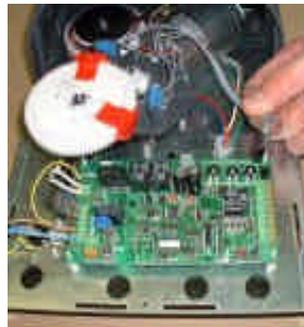
8. Remove limit switch connector.
