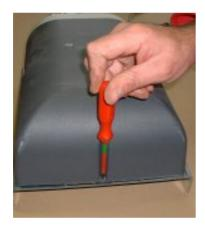
1. Remove retaining screw and flip open the cover.
