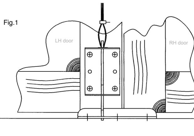
5. Fit the cable stop bracket to the door, pass the cable through it and attach it to the floor bolt using the clamp supplied. close the doors with the motor, then adjust the cable length so that the bottom latch bolt is engaged onto the floor striker plate by **10mm**.
